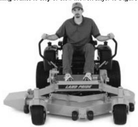
Control Levers in Parking Brake Position Figure 2-4
